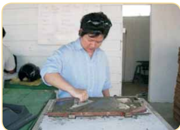
Production of micro concrete roofing tiles in Banda Aceh, Indonesia
