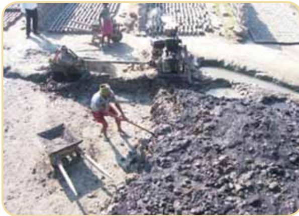
Green brick making with internal fuel in Bangladesh
